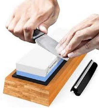
For both side beveled blade: keep on sharpening until you feel the curled metal and then flip the blade and sharpen the other side.
